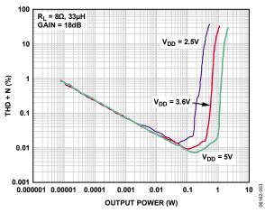
Figure 4. THD + N vs. Output Power into 8  $\Omega$ ,  $A_V = 18 dB$
