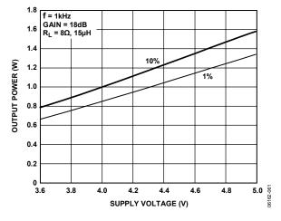
Figure 23. Maximum Output Power vs. Supply Voltage,  $R_L = 8 \Omega$ ,  $A_V = 18 dB$
