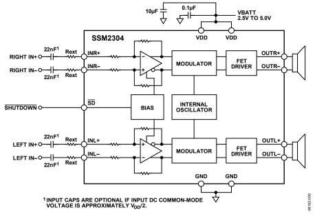
Figure 37. Stereo Differential Input Configuration
