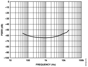
Figure 32. Power Supply Rejection Ratio vs. Frequency
