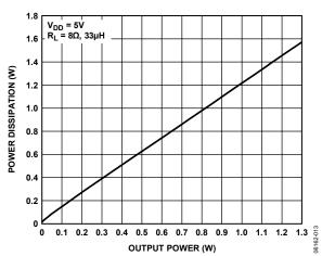
Figure 28. Power Dissipation vs. Output Power at  $V_{DD} = 5.0 \text{ V}$ ,  $R_L = 8 \Omega$
