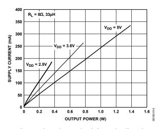
Figure 31. Output Power vs. Supply Current, One Channel
