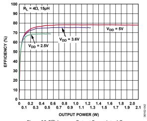
Figure 25. Efficiency vs. Output Power into 4  $\Omega$
