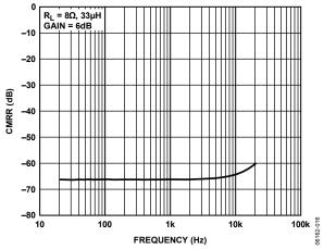
Figure 33. Common-Mode Rejection Ratio vs. Frequency
