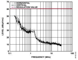
Figure 39. EMI Emissions from SSM2304
