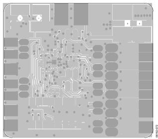
Figure 43. Top Layers Without Top Screen Layer
