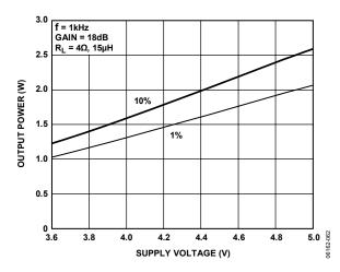
Figure 24. Maximum Output Power vs. Supply Voltage,  $R_L = 4 \Omega$ ,  $A_V = 18 dB$
