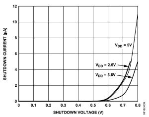
Figure 20. Supply Current vs. Shutdown Voltage
