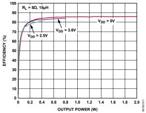
Figure 26. Efficiency vs. Output Power into 8  $\Omega$
