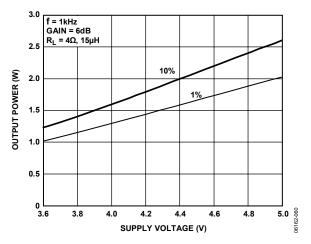
Figure 22. Maximum Output Power vs. Supply Voltage,  $R_L = 4 \Omega$ ,  $A_V = 6 dB$
