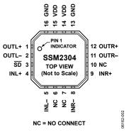
Figure 2. SSM2304 LFCSP Pin Configuration
