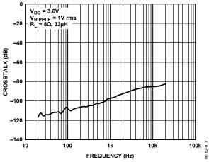
Figure 34. Crosstalk vs. Frequency
