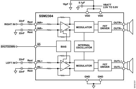
Figure 38. Stereo Single-Ended Input Configuration
