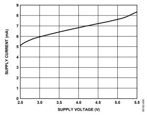
Figure 19. Supply Current vs. Supply Voltage, No Load
